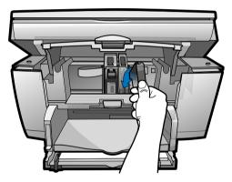
**9** Lower each print-cartridge latch down onto the top of the cartridge, and push down until the latch locks firmly into place.
